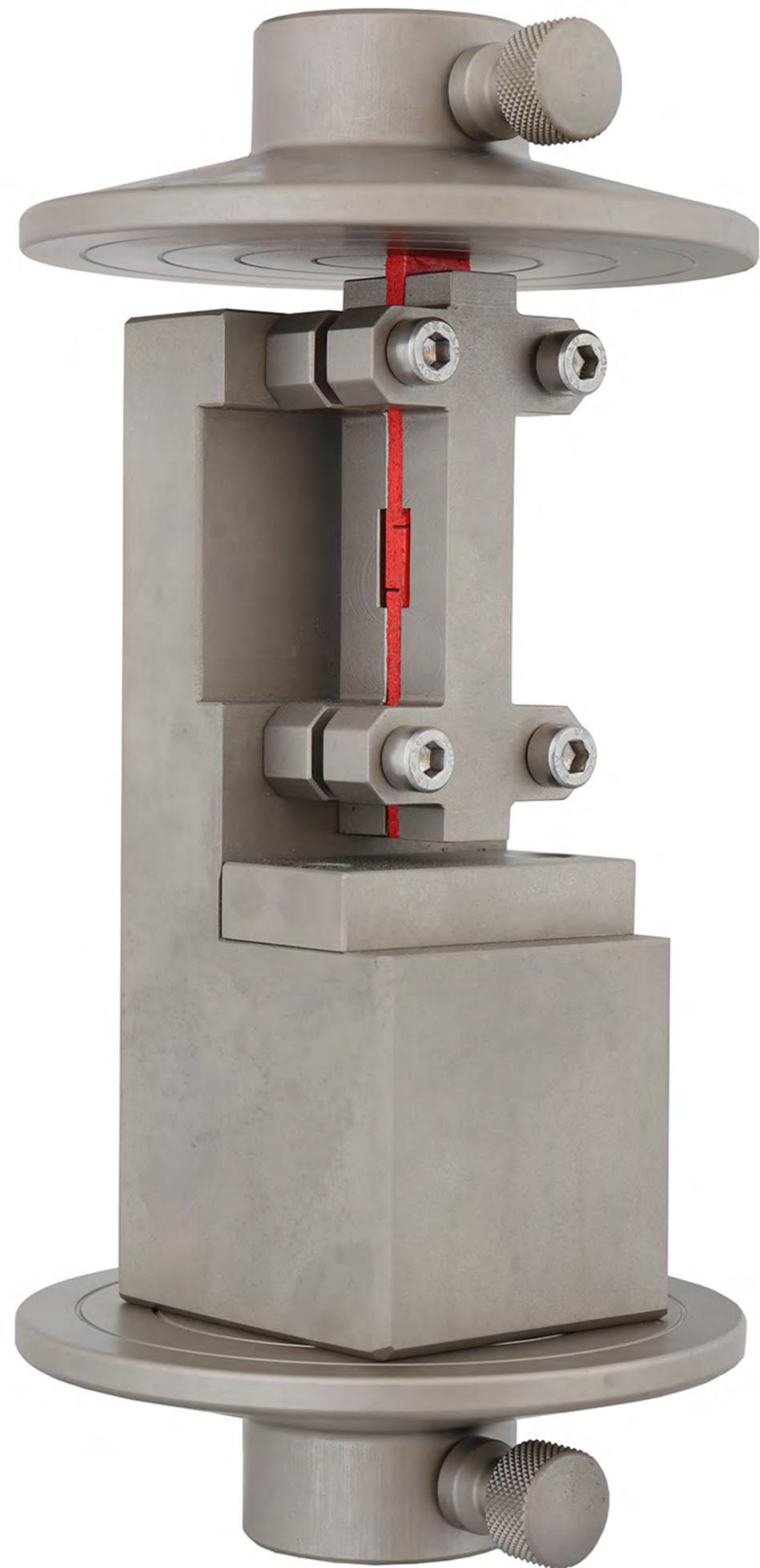
TH23-96 + THS793-GT+E- ASTM-D695-Fig.4 , ASTM-D3846
