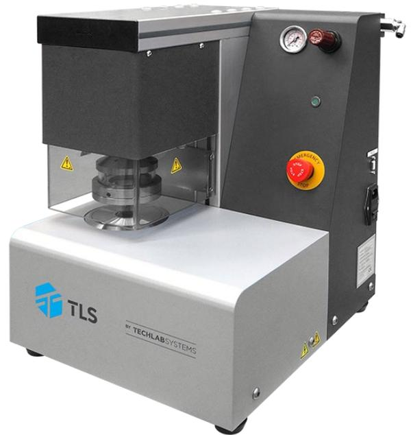
The Testing Software allows Burst Resistance tests to be performed on samples of paper, compact and corrugated cardboard.
