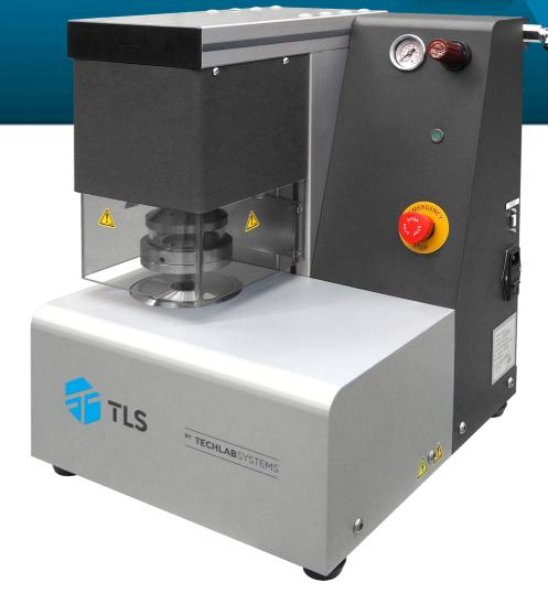
For measuring the bursting strength on materials such as paper, compact and corrugated cardboard "Mullen type"
