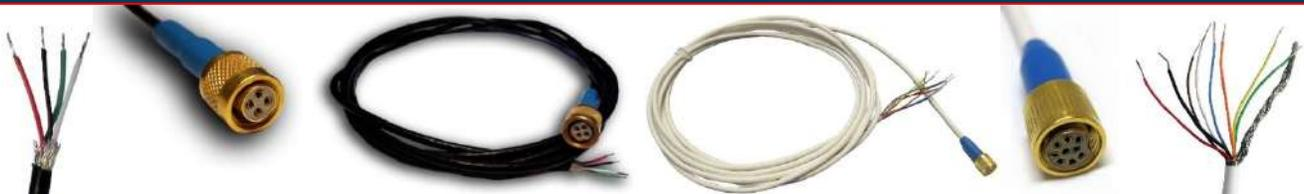
2240: The connector shells, pins and sockets are gold plated brass. The 4PIN-CAB cable consists of four 30 AWG (7x38) silver-plated copper wires with PTFE insulation surrounded by a braided shield. The black FEP shield jacket has a nominal outer diameter of 0.100”.
