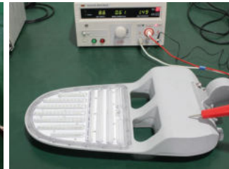
Withstand Voltage Test
