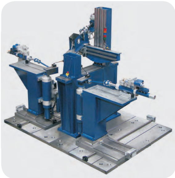
5 DOF durability and characterization steering test machine
