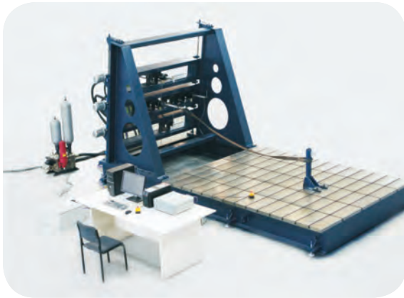
Seatbelt anchorage test machine
