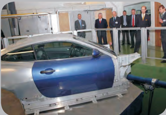
Servotest has delivered a unique low distortion, low noise, long stroke, man rated MAST system
