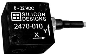
The SDI Models 2460 and 2466 are the triaxial versions of the 2210 and 2260/2266, respectively, rounding out the SDI Universal Module low-cost family. The high performance SDI Models 2470 and 2476 are the three axis versions of the 2220 and 2276 with similarly upgraded SDI accelerometer chips, improved bias and scale factor temperature shift performance, and include an initial calibration certificate.
