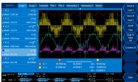
Simultaneous measurement of narrowband and wideband values
