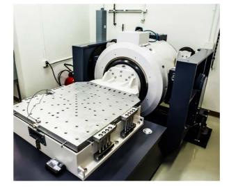
requirements. LST Series slip tables utilize V-groove bearings to guide the magnesium slip plate over an oil-film on a precision ground granite slab. Oil from an integral hydraulic power supply is dispersed through ports in the granite slab under the magnesium slip plate.
