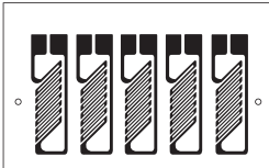
5-element pattern for shearing strain
