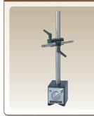
The magnetic stand is used for positioning the sensor. With two joints, laser irradiation can be performed freely. Using it together with the LV-0015 or LV-0016 fine-positioning stage enables fine adjustment of the detecting position.
