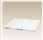
This benchtop vibration isolator does not require compressed air and can be installed anywhere. It isolates the sensor from background vibration transmitted from the floor to improve detection accuracy. The top plate is an SUS plate on which the LV-0030 can be mounted. Outer dimensions: 500 x 600 x 56 mm Maximum load weight : 120 kg Weight : approx. 29 kg Leveling : Hand pump
