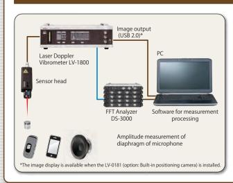
The LV-1800 is the most suitable for measurement of thin film velocity. It can measure the velocity of thin films such as a diaphragm of cell phone's microphone, a corn paper of receiver or speaker, and a transparent film like a liquid crystal display film.
