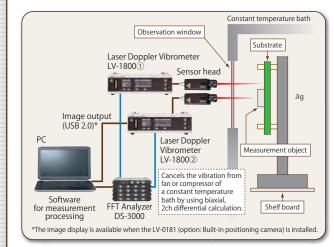
The LV-1800 does not detect transparent objects not located at focal position. Using this characteristic, it can detect vibration of an object inside a vacuum chamber or a constant temperature bath by irradiating laser through a glass or quartz.
