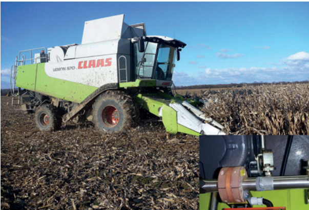
Torque measurement on combine harvester
