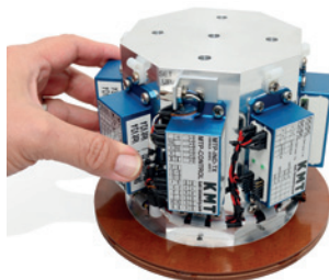
Telemetry for train wheel-set test bench
