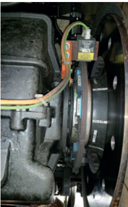
Force measurement on railway wheel set
