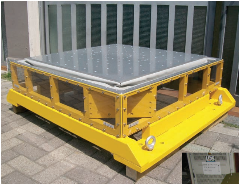
Guided expander 1000x1000 mm with load support armature 440 - 2000 Hz - to be mounted on a trunnion
