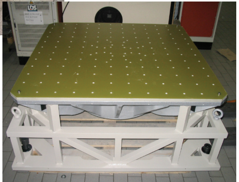
Guided expander 1000x1000 mm with thermal barrier
