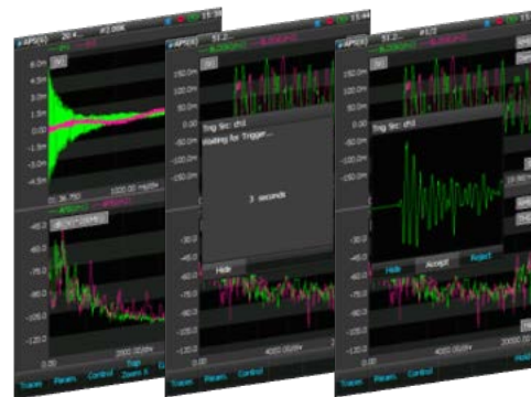
Figure 5: Acquisition Modes 'Free-Run', 'Auto-Trigger', and 'Manual Trigger'
