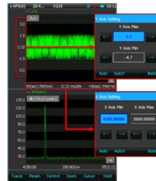
Figure 2: Configure Axis Scaling
