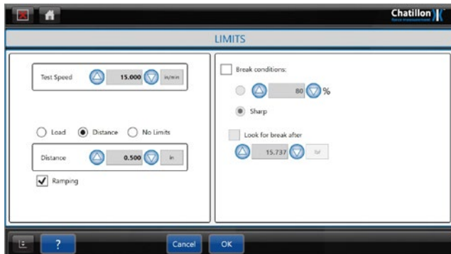
Conduct a quick test by simply entering the type of test, pre-load (if any) and limits.
